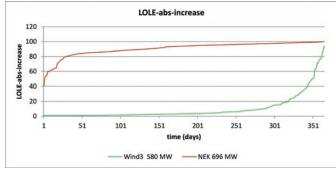
Fig. 8. The LOLE absolute increase factors for the plants in the example power system – nuclear versus wind
