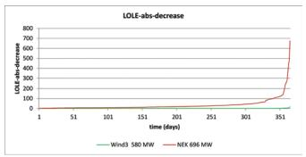
Fig. 9. The LOLE absolute decrease factors for the plants in the example power system – nuclear versus wind
