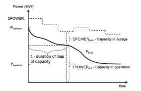
Fig. 3. Graphical representation of parameters for determining improved loss of load expectation
